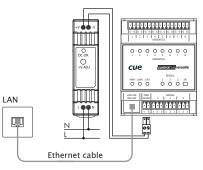
Delivered DIN rail power supply 24 VDC can be used for areas without PoE infrastructure.
