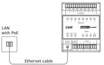
The integrated IEEE 802.3af PoE support allows installation in areas where PoE network infrastructure is installed.
