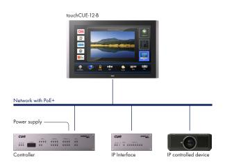
The following diagram describes the use of touch panel with IP interfaces only. This configuration allows to create cost effective distributed control solution where touch panel serves as controller and graphic user interface in one box. In Cue Visual Composer touch panels and controllers are programmed in the same way, which makes possible to use touch panels as fully functional control units.
