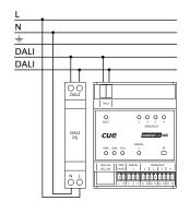
The port does not provide DALI power supply which must be ensured by external DALI power source.
